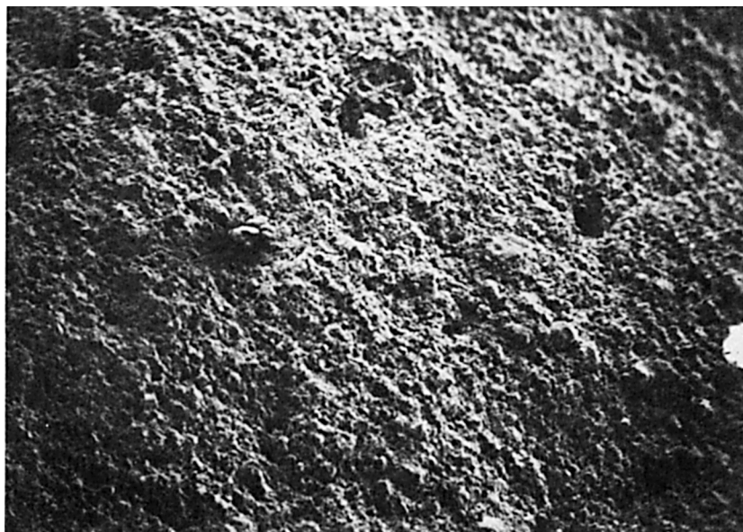
Fig. 2. SEM of ordinary portland cement with SMF dispersant present, showing uniform morphology with no agglomeration.
